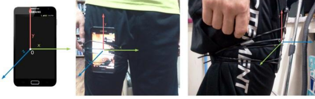
Fig.1. 3-D coordinate of accelerometer and phone attached to the trouser pocket position
