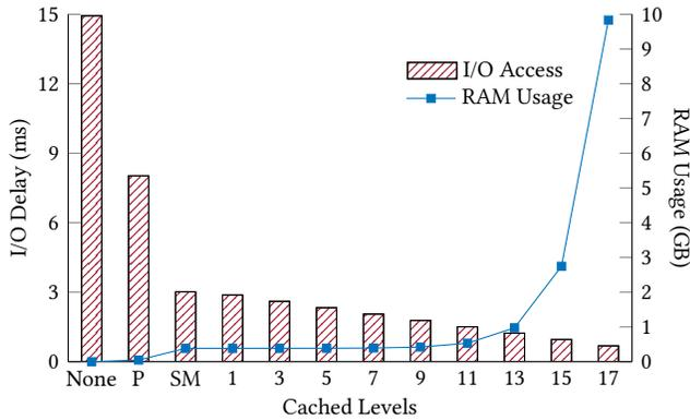
**Figure 7: The impact of caching on the I/O delay and memory usage of MOSE.** “None” denotes no caching; “P” denotes caching the position maps; “SM” denotes caching the stashes and meta-data;  $x$ s-axis represents the catching levels of ORAM trees of EAC and EDB.
